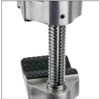
The groove keeps the jaws aligned with one another.
