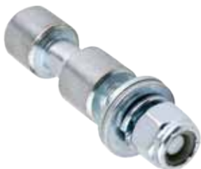
KS-013 Ø17mm Steel Spigot W 80g 2.9oz Ø17mm spigot (DABO) male threaded w/ 3/8"-16 washer & lock nut for C-05 & C-01 family.
