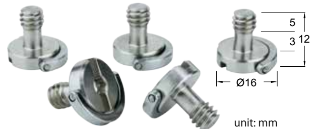
KS-135 unit: mm W 10g 0.35oz 1/4"-20 D-Ring Screw (8mm Shaft length) Kupo 1/4"-20 D-Ring Screw made by chromed steel can be hand-tighten with hinged D-ring or with a screwdriver to the flat head slot. Ideal for quick-release plates or any 1/4"-20 thread compatible device. The shaft is 8mm in length and total length including the head is 12mm. (Set of 5)
