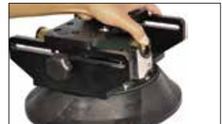
Press the release mechanism to refill air in the evacuated space and then the vacuum cup detaches completely.
