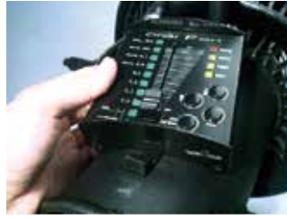
Switch for local or DMX operation mode.
