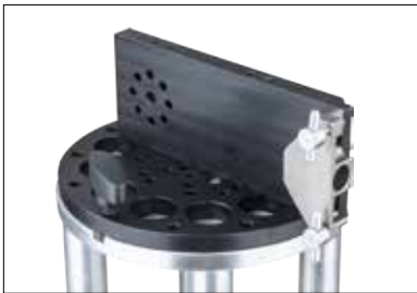
A knob is equipped as key offers a quick adjustment
