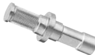
KS-151 Double Stud 16 to 17mm Adapter W 95g 3.36oz Made by solid steel, this double stud features a knurled neck on one side for the maximum friction and one milled flat on the other to avoid rotating while mounted inside a 5/8" baby receiver. Additional 3/8"-16 female threaded is tapped for connecting with a variety of accessories for video and lighting.
