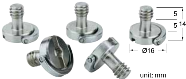
KS-061 unit: mm W 10g 0.35oz 1/4"-20 D-Ring Screw Kupo 1/4"-20 D-Ring Screw made with stainless steel can be hand-tighten with hinged D-ring or with a screwdriver to the flat head slot. Ideal for quick-release plates or any 1/4"-20 thread compatible device. The shaft is 10mm in length and the total length including the head is 14mm. (Set of 5)
