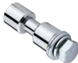
KS-013F Ø17mm Steel Spigot W 75g 2.65oz Ø17mm spigot (DABO), female threaded with 3/8"-16 bolt & washer.
