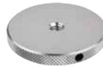
KS-068 Round Knurled 1/4"-20 Female Thread Knob w/ 1.77" (45mm) Flange
